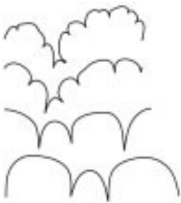
Figure 1. From bottom to top, the computed evolution of a flame expanding in two dimensions reveals the flame shape to be bulges connected by cusps (the cusps point towards the burnt gas side of the flame). The cusp-bulge-cusp shape resembles a cycloid curve.
